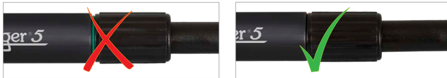
Figure 10-13 Proper Direct Read Cable Connection
