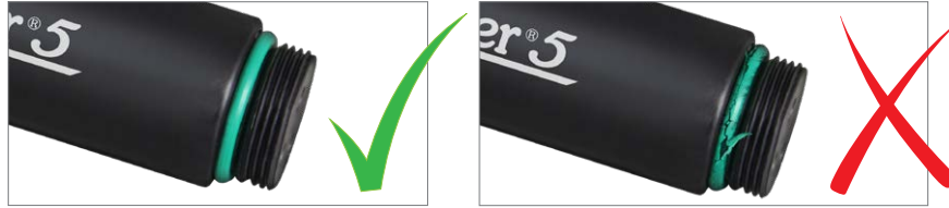
Figure 10-25 Levellogger O-ring Damage
