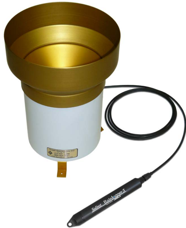
Figure 10-21 Rainlogger 5 Connected to Tipping-bucket
